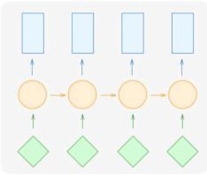
Multiple data inputs and multiple data outputs
