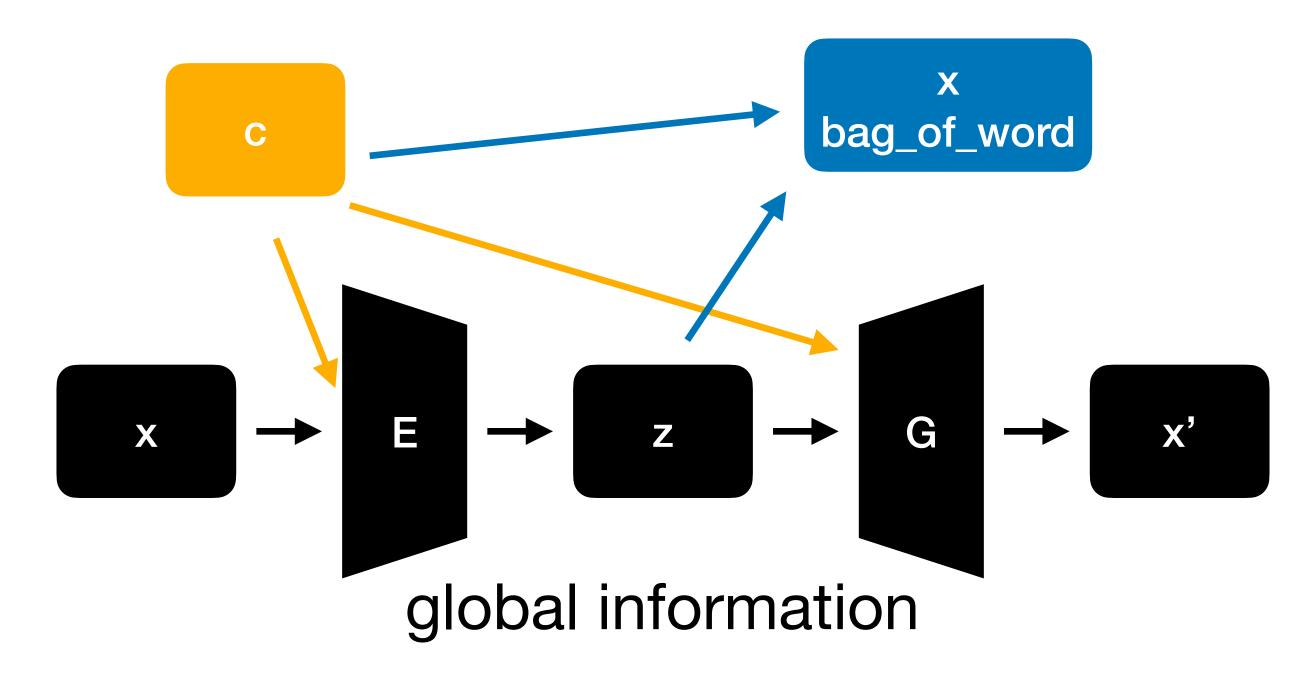
$$\mathcal{L} = E_{z \sim Q(x,c)}[\log P(x \mid z,c)] - \lambda \mathcal{D}[Q(z \mid x,c) || P(z \mid c)] + \mathcal{L}_{bow}$$
